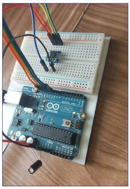
Quick tutorial showing how to program the ATtiny85 from the Arduino IDE with the help of the Arduino Uno!
